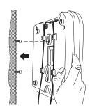
7. Plug the other end of the telephone line cord into the wall jack.
